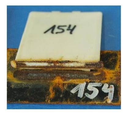
The laser structuring destroys the KTL coating, leading to corrosion and loss of adhesion
